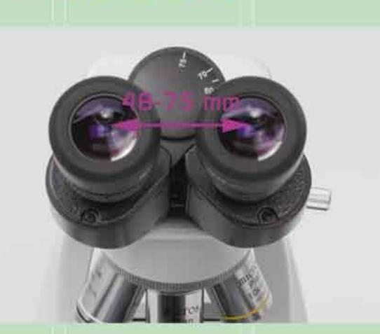
With the ARCTYPE tube the eyepieces can be positioned in two different heights. The eyepoint adjustment range is 350 - 395 mm, which means small and tall users can have an ergonomic and relaxed posture while observing. The interpupillary distance adjustment (48 - 75 mm) and the diopter adjustment ensure that the microscope easily fits to every user.
