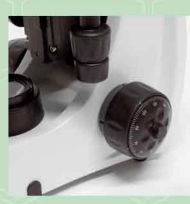
The ergonomic arranged coaxial coarse and fine focus controls are located on the left and the right side of the microscope base. Along with the focusing controls, Petunia also features a built in tension adjustment - which controls the mobility of the coaxial coarse - and an Auto Focus Stop Unit Function - which prevents a collision of objective and specimen to avoid possible damage of both. Total focusing range is 20 mm and the graduation reading on the right fine focus is 2 \mu per division.
